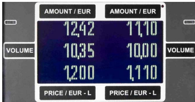
Fig. 4 - Mask of the display unit with graphic display, electromechanical totalizers and preselecting keyboards
